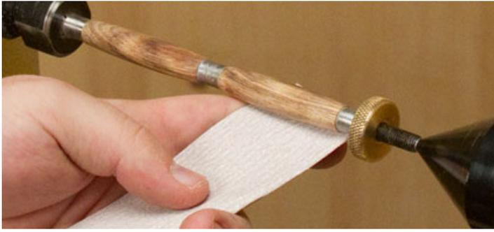
7. Move the tool rest away from blanks and sand the blank through 320 grit then final sand with steel wool.
