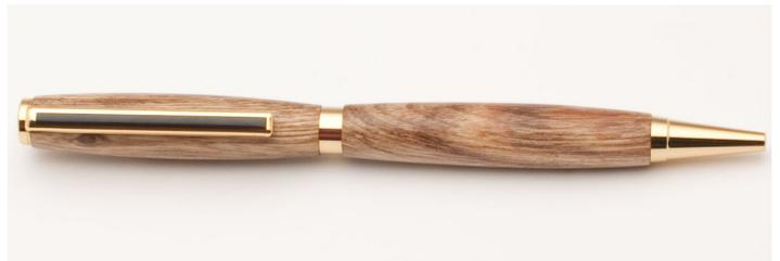
5. Slide the center band over the twist mechanism. Slide the clip/cap barrel over the exposed twist mechanism to complete the pen.
