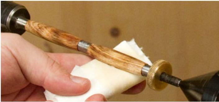
8. With the lathe stopped, apply the first coat of finish. Turn the lathe on and with light pressure buff the blank with the rag. Repeat until desired gloss is achieved. Apply a small amount of wax to a small rag and lightly buff the blanks to a final finish.
