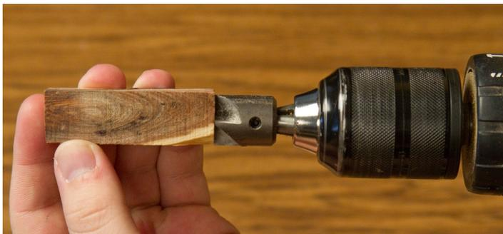
3. Trim the ends of the pen blanks using a barrel trimmer. This squares the ends of the blank to the center of the tube assuring a proper fit during assembly.
