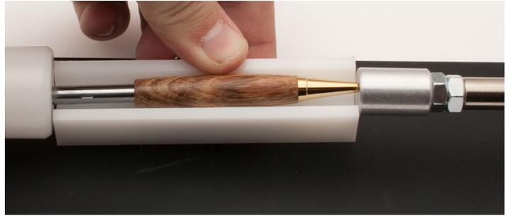
3. Start the twist mechanism, brass end first, into the opposite end of the writing tip. Lay the assembly parts into the vee groove of the Pen Press Block and press the parts together until the block stops the parts from pressing together any further.
