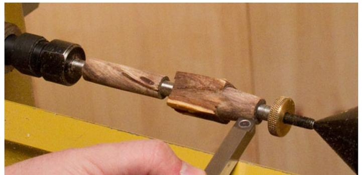
5. Turn the corners off the blank with the Mini Easy Rougher. Start at one end of the blank and work toward the center a cutter-width at a time. Turn both blanks down to a cylinder about 1/8" larger in diameter than the pen bushings.
