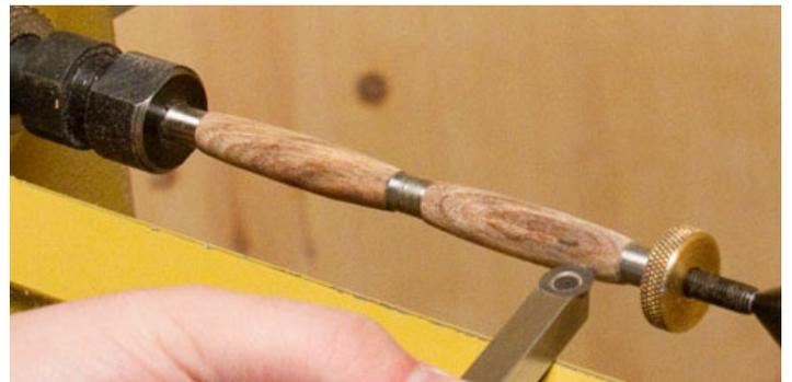
6. Turn the blanks to the finished shape and diameter with a the Mini Easy Finisher. Taper the blank in the direction bushing on each end of each blank, leaving the center slightly thicker.
